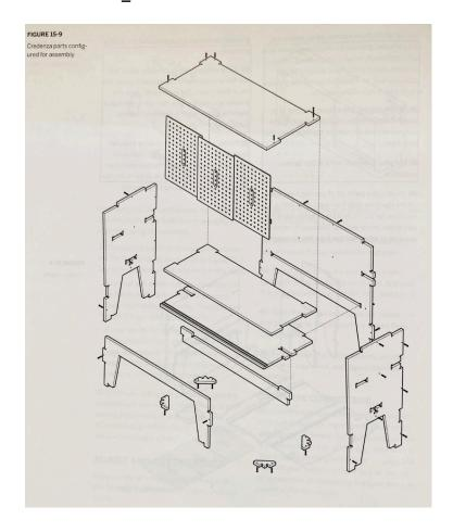
**Process:** CNC Router (subtractive fabrication)
