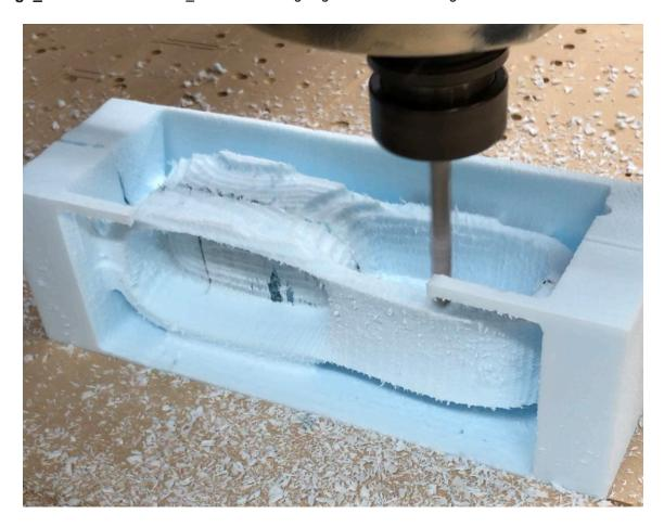
**Process:** CNC Router (subtractive fabrication)
