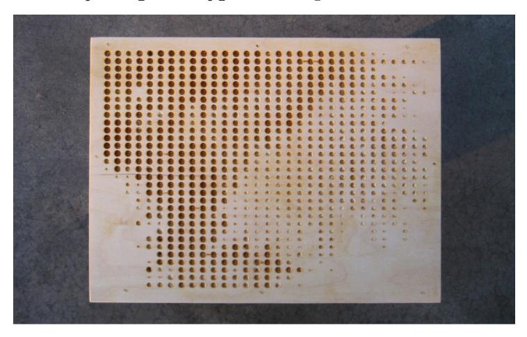
**Process:** CNC Router (subtractive fabrication)
